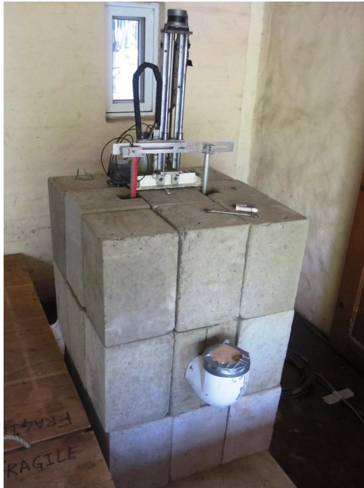
Figure 3: Experimental set up. Concrete blocks surround one of the duct samples. On top is THATIR's driving mechanism that moves down the tubes containing the detector (in red) and the source (in white) on each side of the duct.
